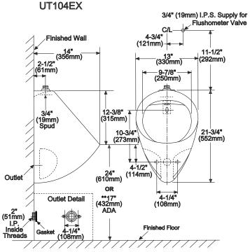
\*\*Recommended for ADA height installation for 17" floor to rim.
