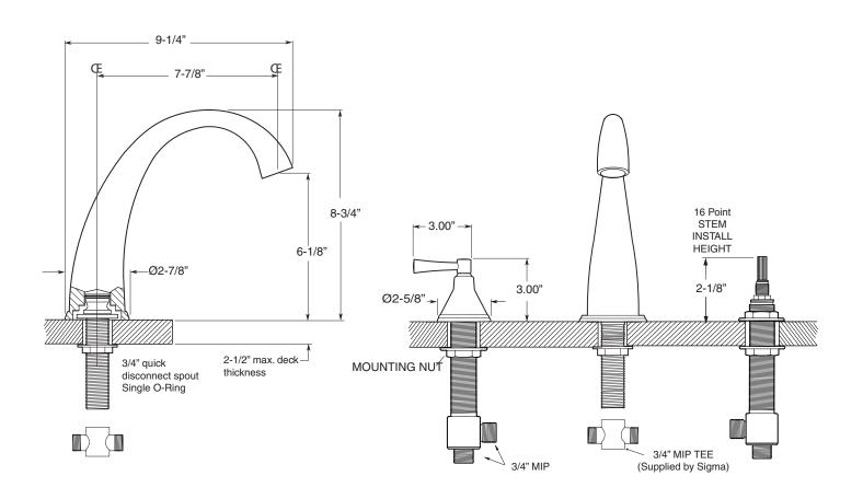
NOTE: Spout and valves install through 1-1/4" diameter holes.
