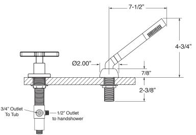
Spout and valves install through 1-1/4" diameter holes. Plumber to provide 3/4" supply lines to valves
