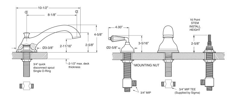
NOTE: Spout and valves install through 1-1/4" diameter holes. Plumber to provide 3/4" supply lines to valves
