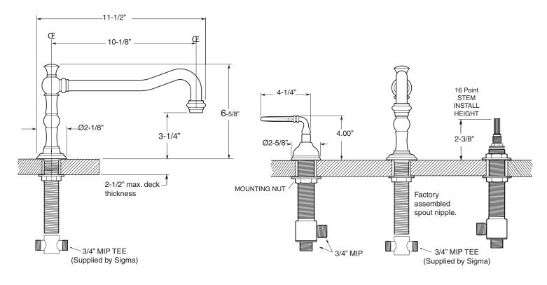
NOTE: Spout and valves install through 1-1/4" diameter holes. Plumber to provide 3/4" supply lines to valves
