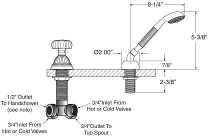
Spout and valves install through 1-1/4" diameter holes. Plumber to provide 3/4" supply lines to valves
