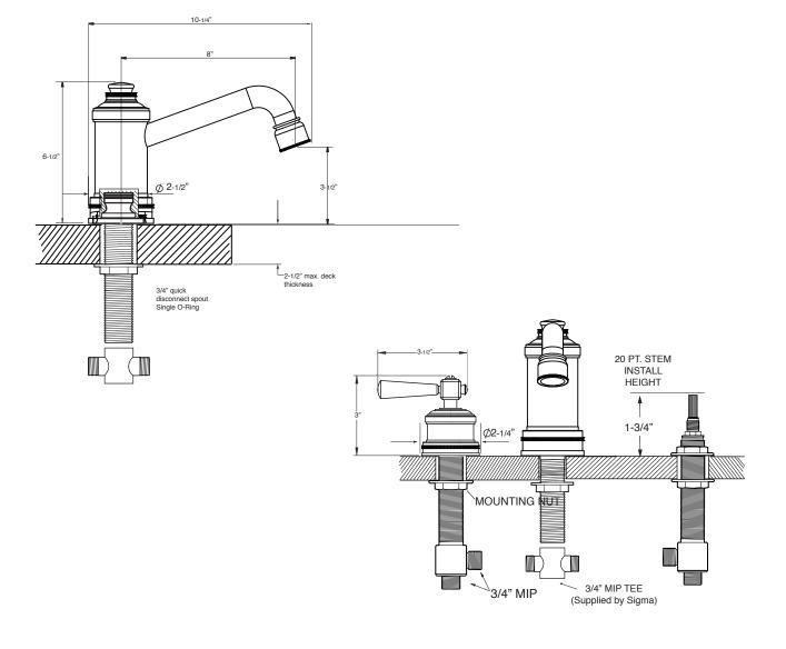
NOTE: Spout and valves install through 1-1/4" diameter holes. Plumber to provide 3/4" supply lines to valves
