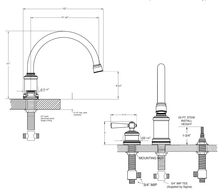
NOTE: Spout and valves install through 1-1/4" diameter holes. Plumber to provide 3/4" supply lines to valves
