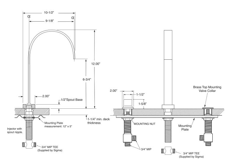
NOTE: Spout and valves install through 1-1/4" diameter holes.
