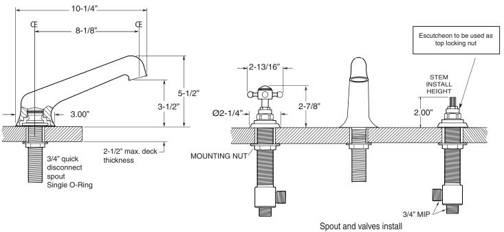
through 1-1/4" diameter holes. Plumber to provide 3/4" supply lines to valves 8-1/4" 5-3/8" NOTE: 1/2" outlet for in-line vacuum breaker Ø2.00"-(18.15.055), and 60" chrome spiral hose (18.10.016) - INCLUDED 7/8" 2-3/8" 1/2" Outlet To Handshower 3/4"Inlet From (see note) Hot or Cold Valves 3/4"Inlet From 3/4"Outlet To Hot or Cold Valves **Tub Spout**
