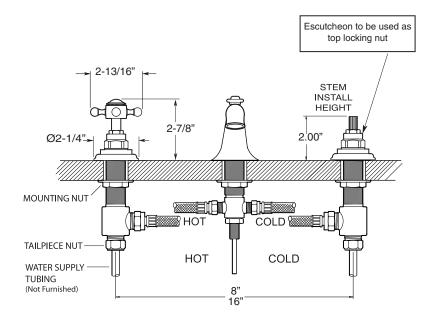
NOTE: Spout and valves install through 1-1/4" diameter holes
