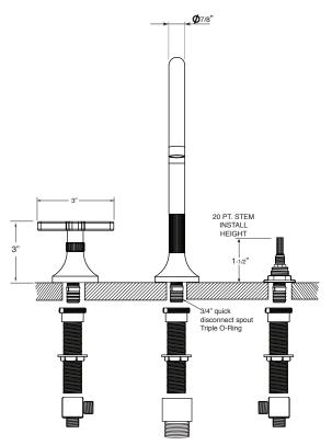
Spout and valves install through 1-1/4" diameter holes. Diverter valve installs through 1-1/2" diameter holes. Plumber to provide 3/4" supply lines to valves
