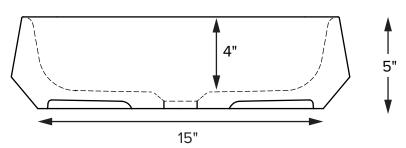
Base dimensions on counter top: 5" in diameter Always measure sink on-site to ensure cut-out accuracy.
