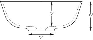
Base dimensions on counter top: 5" in diameter Always measure sink on-site to ensure cut-out accuracy.
