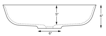
Base dimensions on counter top: 5" in diameter Always measure sink on-site to ensure cut-out accuracy.
