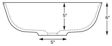
Base dimensions on counter top: 5" in diameter Always measure sink on-site to ensure cut-out accuracy.
