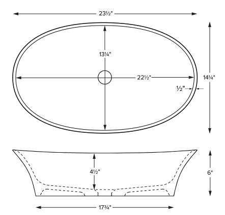
Base dimensions on counter top: 173/4" x 103/4" Always measure sink on-site to ensure cut-out accuracy.
