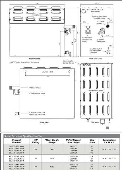
\*Refer to sizing guidelines to accurately determine the proper size generator for the installation. 90 °C copper wire is required for generator connection. Installation shall be in accordance with NEC and local electrical codes.
